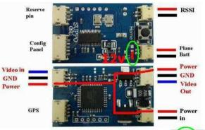
Jumper solder to 12V Power in --- Vin Vcc ---- Vout vcc are direct connected
