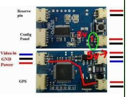
Jumper solder to 5V Vout vcc get 5V fixed and Power in---Vin Vcc are direct conne
